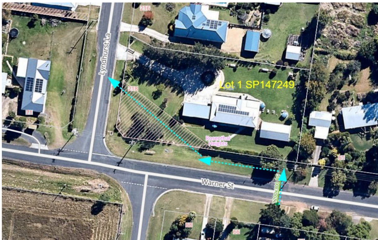
Fig 1: Drainage Flow on Lot 1 SP147249
