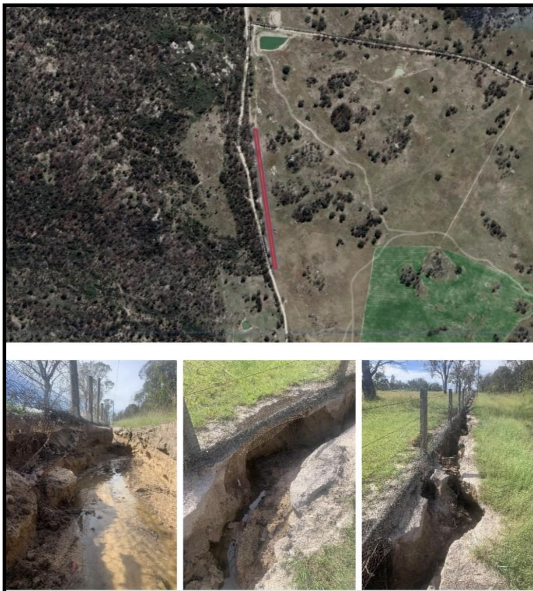
Plate 1. Location and indicative images of the scouring along the rabbit fence near Dalveen.
