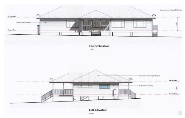
Figure 5: Proposed front and side elevations
